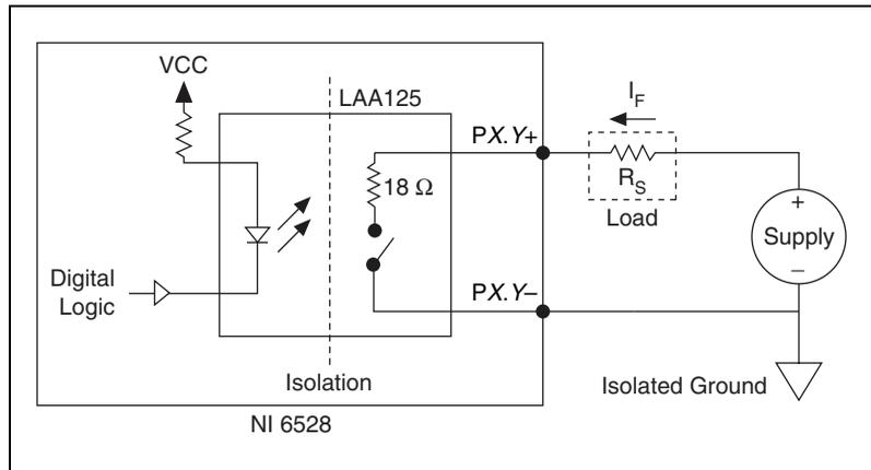
**Figure 6.** Sinking Current Connection Example
