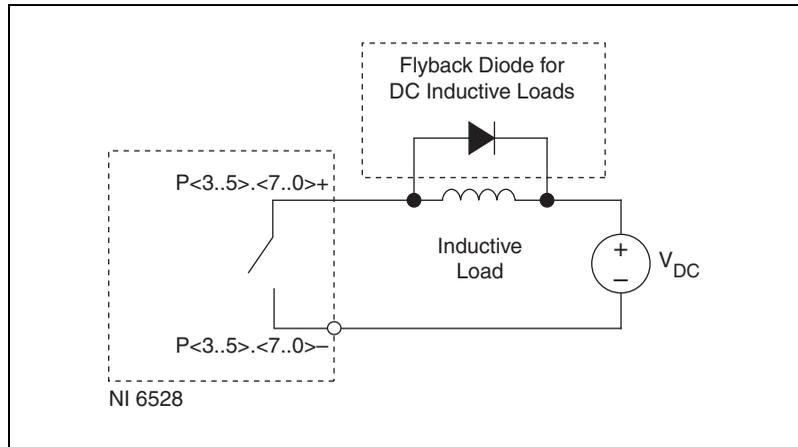
**Figure 9.** Limiting Flyback Voltages at the Inductive Load
